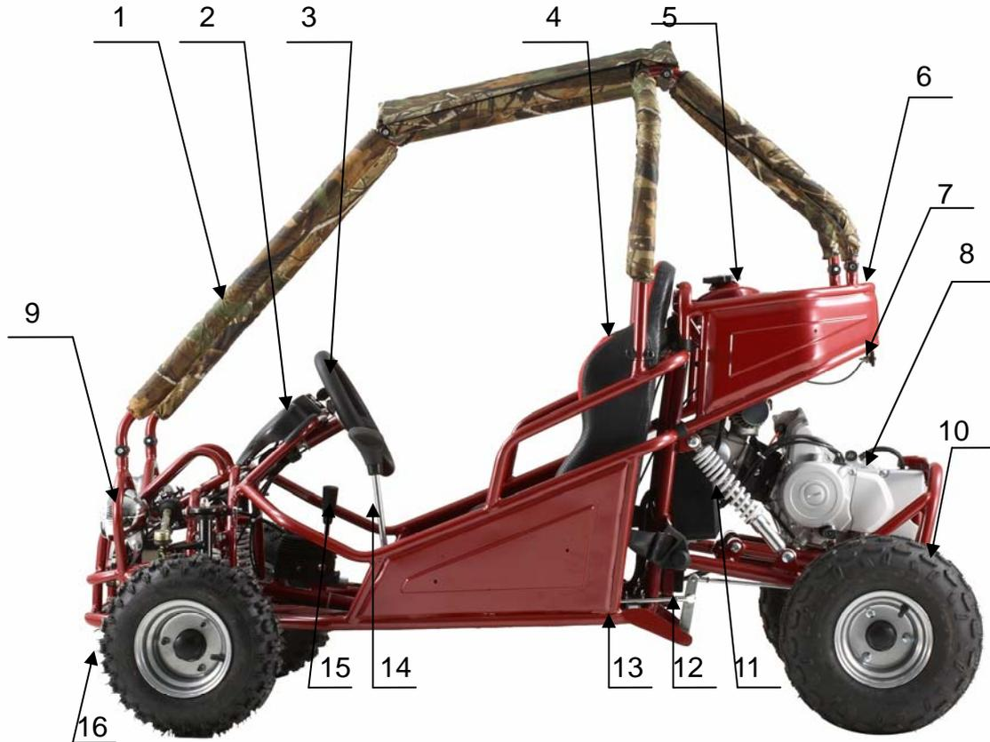
1.TOP SAIL FRAME 2.METER 3.STEERING WHEEL 4.SEAT 5.OIL TANK 6.REAR RACK
