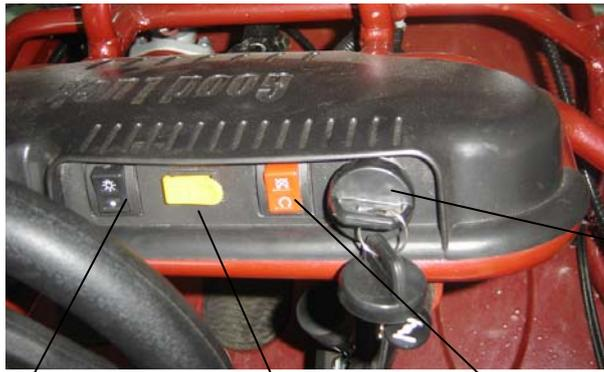
Headlight switch    Horn switch    Stop switch
